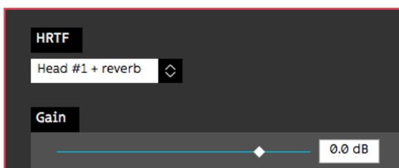
The [Render Hoa2Bin] plugin can be inserted in a DAW as a spatial effect with 4, 9, 16, or 25 inputs and 2 output channels. The input is a Higher Order Ambisonics signal up to order 4, using the ACN/SN3D (ambiX) convention. The output is a binaural signal for headphones. Several HRTF sets can be selected, with or without reverberation.
