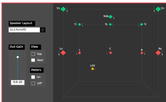
The [Render Hoa2Spk] plugin can be inserted in a DAW as a spatial effect with 4, 9, 16, or 25 inputs and 32 output channels. The input is a Higher Order Ambisonics signal up to order 4, using the ACN/SN3D (ambiX) convention. The output is a multichannel signal adapted to the selected loudspeaker layout. Several output loudspeaker layouts are supported, ranging from stereo to 30.2.
