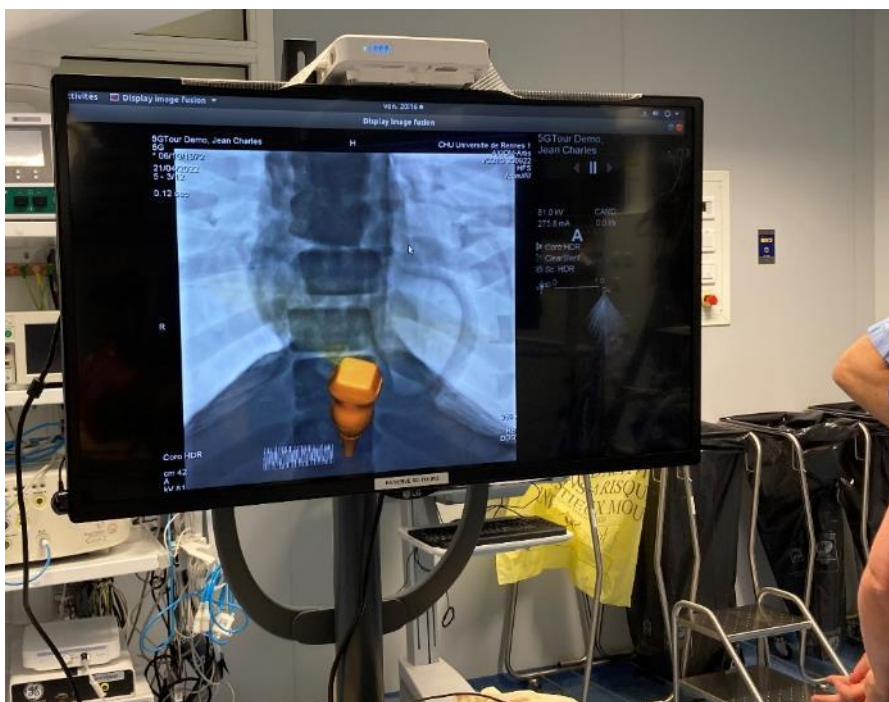
Ultrasound and X-ray signals are merged by the augmented reality application and transmitted over the 5G network ©b<>com
